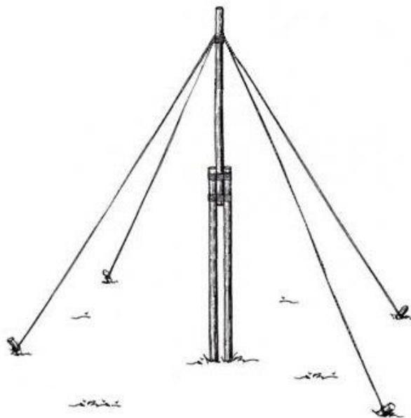
First choose an open area away from overhead power lines. Using rope, lash poles together to gain extra height. Attach additional ropes near the top of the mast, which will be used to guy the mast.
